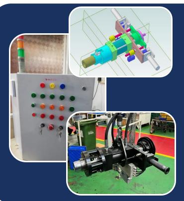
Oil Seal Pressing Unit Poka Yoke using PLC Control Panel for Engine Assembly Line in Engine Manufacturing MNCs
