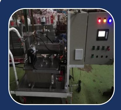
Engine Coolant Temperature Conditioning Unit using PLC HMI based Control Panel for Engine Testing in Automobile MNC
