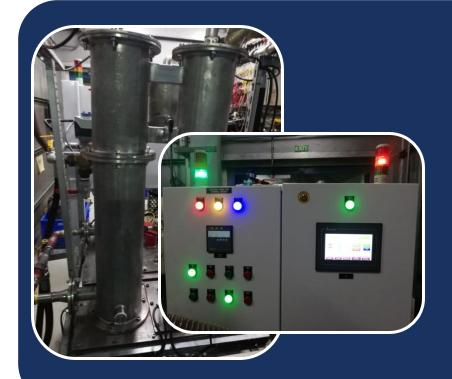
PLC HMI based Control Panel for Engine Coolant Temperature Thermal Shock Unit for Engine Testing in Automobile MNC
