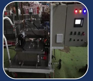
Engine Coolant Temperature Conditioning Unit using PLC HMI based Control Panel for Engine Testing in Automobile MNC
