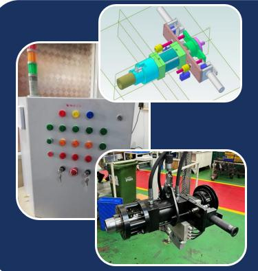
Oil Seal Pressing Unit Poka Yoke using PLC Control Panel for Engine Assembly Line in Engine Manufacturing MNCs
